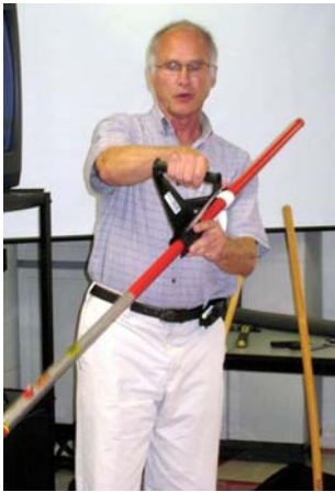
Kirk Ballin, VA Agrability, demonstrates a "D" handle that makes tool use easier on backs.
